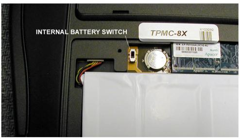
**TPMC-8X Internal Battery Switch**
